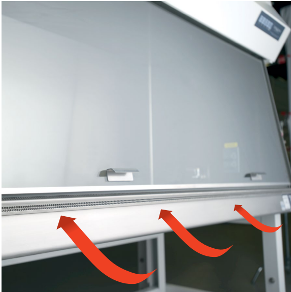
ReadySAFE™ mode – Unique bypass armrest allows cabinet to continue operation with closed viewscreen
