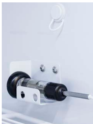
Temperature sensor in glycol bottle
